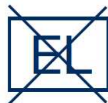
Lamp not suitable for emergency operation
